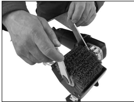
Fig. 3: Brush drum replacement
